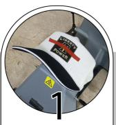
Preheat the cap to 320 °F (160 °C) for 10 seconds and use a heat-resistant tape for patch placement where needed
